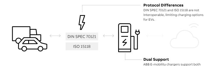
Traditionally, EV to EV charger communication is covered by two standards: DIN SPEC 70121 and ISO 15118. DIN SPEC 70121 is more prevalent in the field because it was published earlier than the current version of ISO 15118-2, but ISO 15118-2 has much richer capabilities, including 'Plug and Charge', encryption, and digital certificates.
