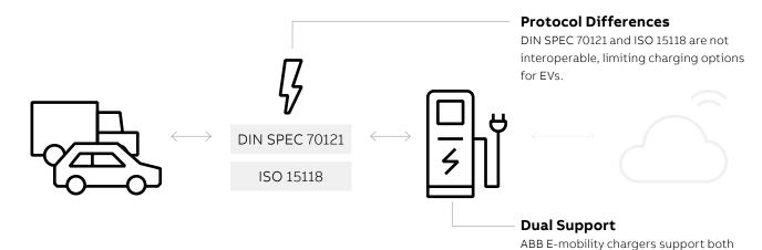
Traditionally, EV to EV charger communication is covered by two standards: DIN SPEC 70121 and ISO 15118. DIN SPEC 70121 is more prevalent in the field because it was published earlier than the current version of ISO 15118-2, but ISO 15118-2 has much richer capabilities, including 'Plug and Charge', encryption, and digital certificates.
